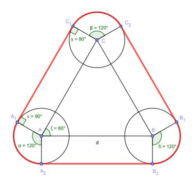
The belt wraps around all three pulleys, hence the part of the belt connecting any two pulleys is tangent to them. Let's drop radii to the points of tangency. Without loss of generality, consider the quadrilateral  $AA_1C_1C$ . Then the angles  $\angle AA_1C_1 = \angle CC_1A_1 = 90^\circ$ , and since  $AA_1 = CC_1 = r$ , it follows that  $AC = A_1C_1 = d$ . Similarly,  $C_2B_1 = A_2B_2 = d$ .
