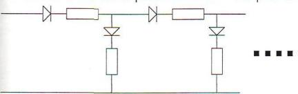
The current through the last section is  $l_0$ . Find the current through the whole circuit and voltage on it.
